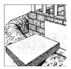
**RIGID INSULATION** is made from fibrous materials or plastic foams and is pressed or extruded into board-like forms and molded pipe-coverings. These provide thermal and acoustical insulation, strength with low weight, and coverage with few heat loss paths. Such boards may be faced with a reflective foil that reduces heat flow when next to an air space.
